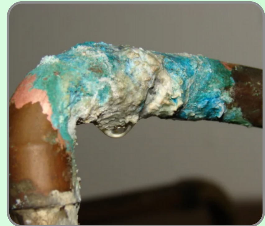
Green coating on copper
