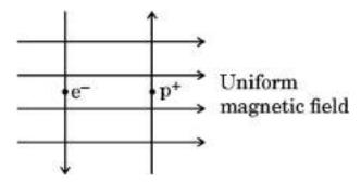
A uniform magnetic field exists in the plane of paper as shown in the diagram. In this field, an electron (e<sup>-</sup>) and a positron (p<sup>+</sup>) enter as shown. The electron and positron experience forces:
